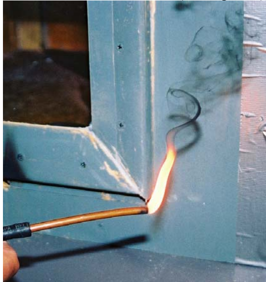
Figure 4 – Smoke Source, 2” laminar MAPP Gas flame
