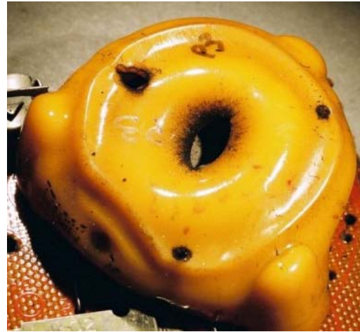
Figures 13 a. and b. – Patterns Persistence Soot agglomeration on a horn enclosure central sound exit opening before (left) and After (right) heating to 433° F. (223° C) for thirty minutes
