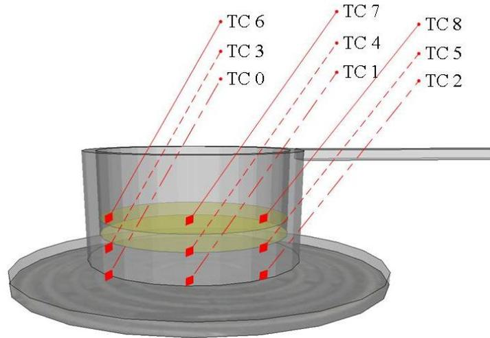
Figure 17: TC placement for canola oil and vegetable oil
