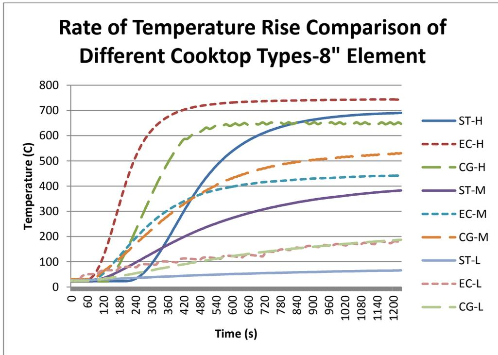
Figure 24: Rate of Temperature Rise-Cooktop Type Comparison (8" diameter heating element)
