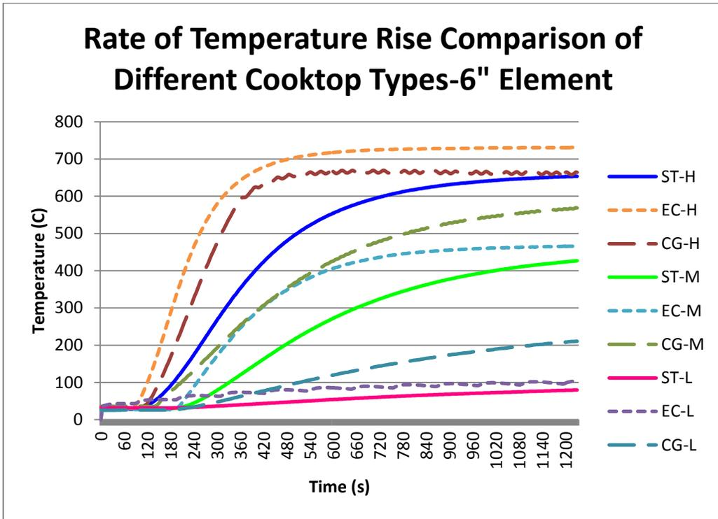
Figure 23: Rate of Temperature Rise-Cooktop Type Comparison (6" diameter heating element)
