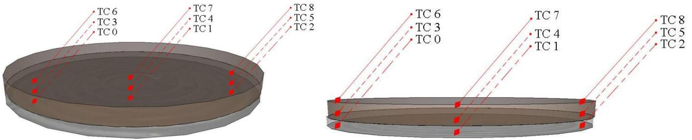
Figure 14: TC placement for corrugated paper (cardboard box): (left) isometric view; (right) elevation view
