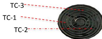
Figure 21: TC location for rate of rise temperature measurements
