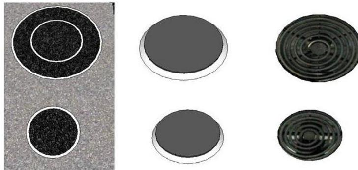
Figure 4: Three types of cooktop elements (left) ceramic-glass, (center) Safe-T-element over coil, (right) coil element
